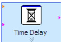
2. **Time Delay** from **Functions->Programming->Timing** palette.
